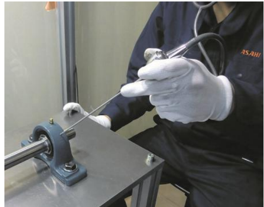
Photo 6.1: Checking the rotation noise with a listening rod
