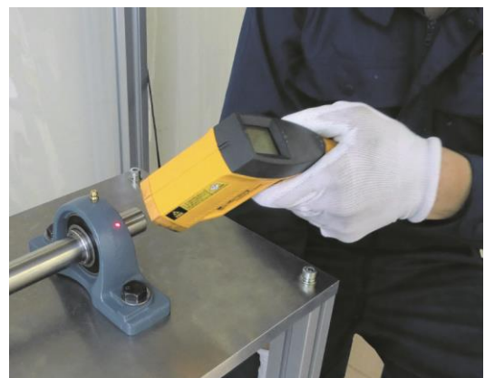
Photo 5.3: Temperature measurement (non-contact type)
