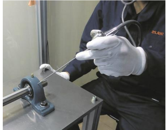
Photo 5.1: Checking the rotation noise with a listening rod
