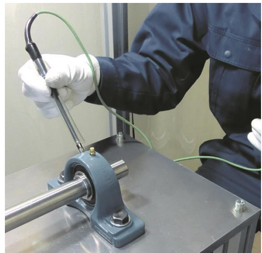
Photo 5.2: Temperature measurement (contact type)
