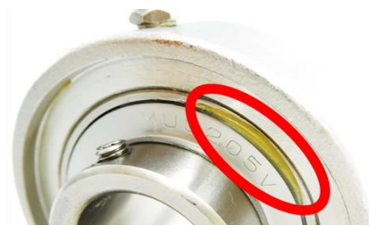
Photo 7.3: Normal grease discharging conditions from inside the bearing
