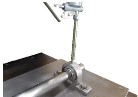
Photo 7.2: Example of filling with a grease gun
