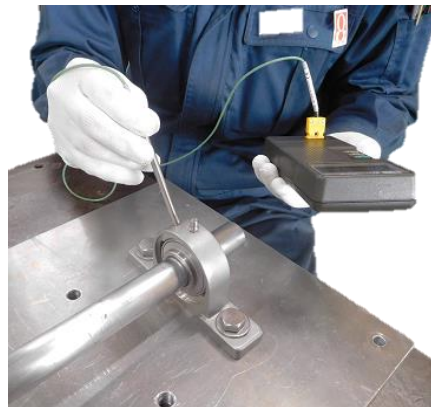
Photo 6.2: Temperature measurement (contact type)
