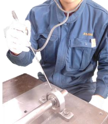
Photo 6.1: Checking the rotation noise with a listening rod
