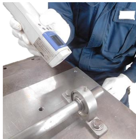
Photo 6.3: Temperature measurement (non-contact type)
