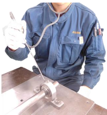
Photo 6.1: Checking the rotation noise with a listening rod
