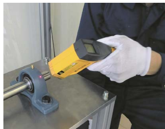
Photo 7.3: Temperature measurement (non-contact type)
