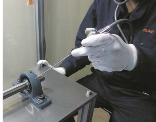
Photo 7.1: Checking the rotation noise with a listening rod
