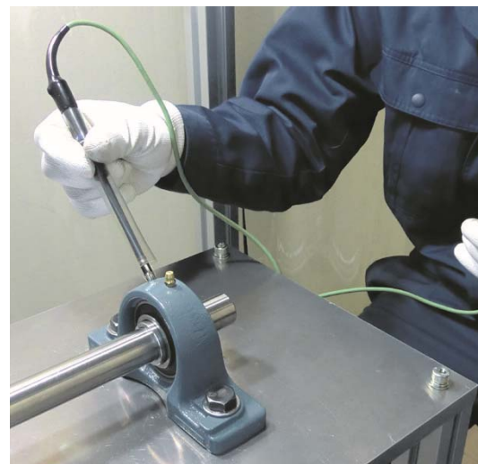
Photo 7.2: Temperature measurement (contact type)
