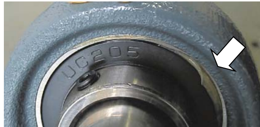
Photo 8.3: Normal grease discharging conditions from inside the bearing
